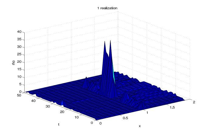
Temporary overload of the bottleneck located at x = 1.
