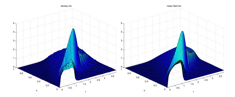
Influx F(x = 0) temporarily at  $2.0 \times$  the bottleneck capacity Left: 500 realizations, Right: mean field equations
