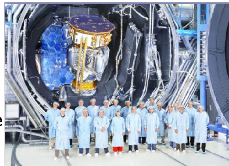
LPF transfer orbit thermal testing
