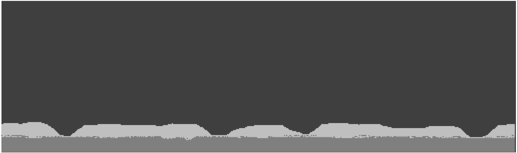
Figure 3: Germanium on Silicon - 16 monolayers. 600^{\circ}K , 1 monolayer per second. (Si-Ge bond energies 30% greater than Si-Si or Ge-Ge bonds)
