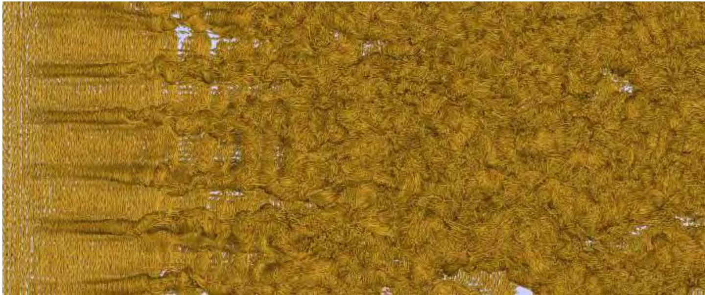
Transition is dominated by the appearance of vortex furrows - spaced approximately at the boundary layer thickness.
