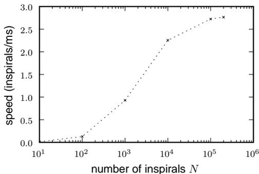
FIG. 1: Performance of the GPU card. We vary the number of inspirals  $N$  scheduled simultaneously on the GPU. For fewer than 100,000 inspirals peak performance is not reached, as there are not enough simultaneously executing threads to mask memory access latency. At 100,000 inspirals saturation is reached as the GPU works serially through the extra inspirals.
