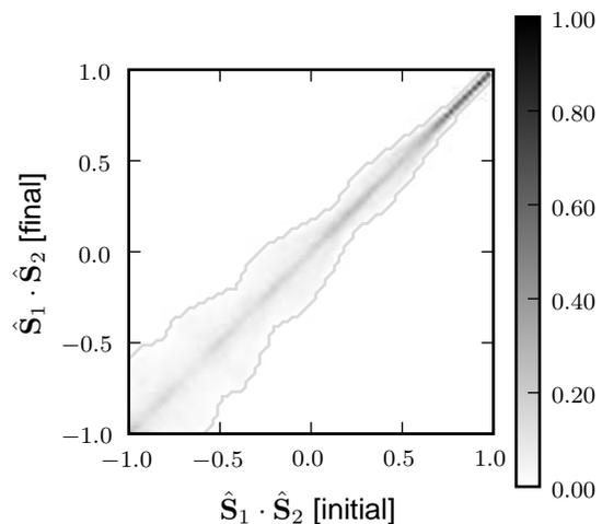
FIG. 4: Final versus initial spin scalar product  $\hat{\mathbf{S}}_1 \cdot \hat{\mathbf{S}}_2$ . The plot shows a high correlation in the scalar product between initial and final scalar product for the equal mass ( $m_1 = m_2 = 0.5$ ), maximally spinning ( $\chi_1 = \chi_2 = 1$ ) case. In light gray we show the 0-contour line to make it easier to see how far the configurations have spread.
